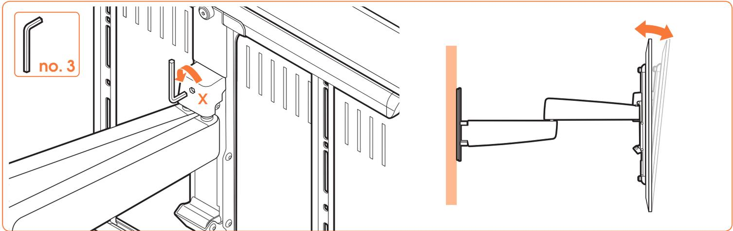
● **For tilt correction, adjust screw X.**
