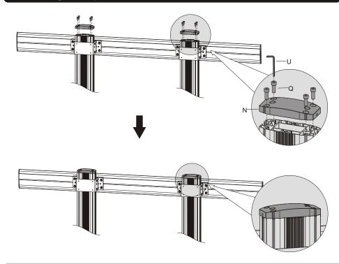
Attach the top covers to the columns using the appropriate screws. Tighten all screws with an Allen key.
