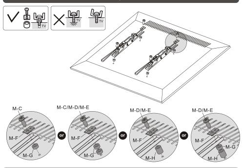
Note: Choose the appropriate screws, washers and spacers (if necessary) according to the type of screens.
