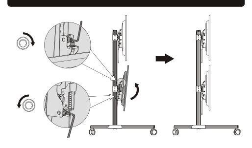
If the displays tilted down, rotate the adjustment screws as shown in figure.
