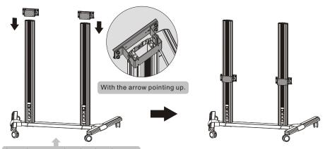
Insert the support plates into the columns along the column rails respectively.
