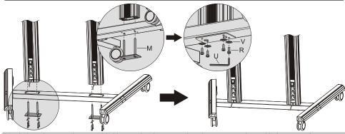
Attach the columns to the assembled base using the connecting pieces, secure them with the appropriate screws. **NOTE:** Lock the brakes on the casters to avoid any sudden movements during installation.
