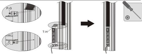
Attach the power sockets to the back of columns using the appropriate screws. Tighten all screws with a phillips screwdriver.
